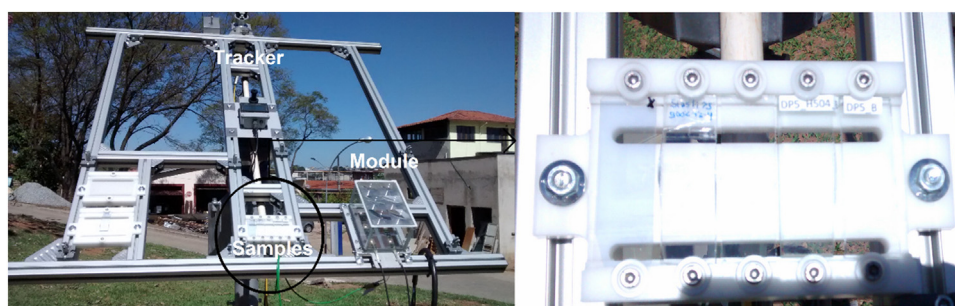
Fig. 1. Soiling test facility: solar tracker (left) and the sample holder (right).
